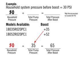
Based on this example, the recommended model for this application is the 18035R020PC1.
